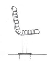
Surface mount: 2 1/2" squared steel tube welded to 3/8" x 4" x 9" base plate with holes for two 1/2" anchor bolts 7" apart.
