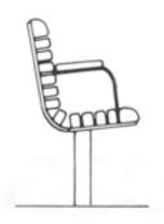
Armrest available for most benches.  $3/16" \times 2"$  formed steel plate is welded to the bench frame and supports  $2" \times 3"$  wood arm.
