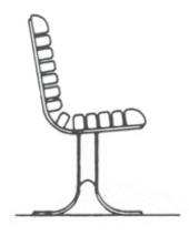
Portable base:  $3/8" \times 2 1/2"$  formed steel continuous welded to  $3/8" \times 2 1/2"$  stiffener plate between legs.
